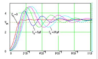
But, add a single 5-pF load to the end of that same trace, and it will begin to ring, taking an extra 2 ns to settle to within acceptable voltage margins after each transition.
